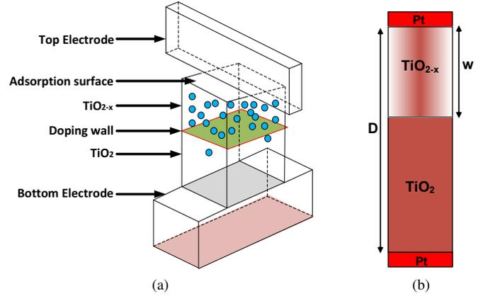
Fig. 1. (a) Structure of memristor for sensing applications. Both sides of the top contact is left uncovered to enhance interaction of target gas with the titanium oxide layer (b) Structure of the  $TiO_2$  based memristor fabricated by HP Labs.
