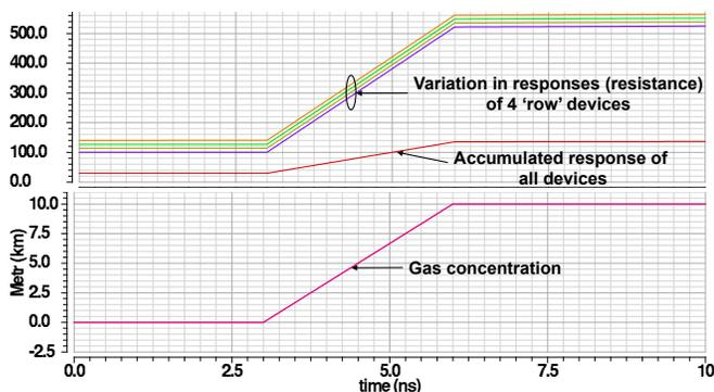
Fig. 4. Simulation result of exposing a row from a  $4 \times 4$  memristor crossbar array to a range of gas concentration.
