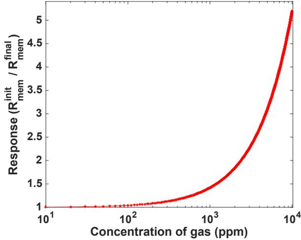
Fig. 2. Sensor response to different concentrations of an oxidising gas.  $R_{mem}^{init}$  is calculated using Eqn. 2 with the initial values of  $R_{on}$ ,  $R_{off}$ .  $R_{mem}^{final}$  (Eqn. 3) is the memristance of the sensor after gas interaction, where  $R_{on}$  changes to  $R_{on\_eff}$ .
