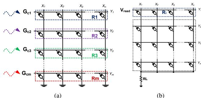
Fig. 3. (a) An  $m \times n$  array of multiple sensors able to detect  $m$  different gases. (b) Reading technique for the multi-sensing structure.
